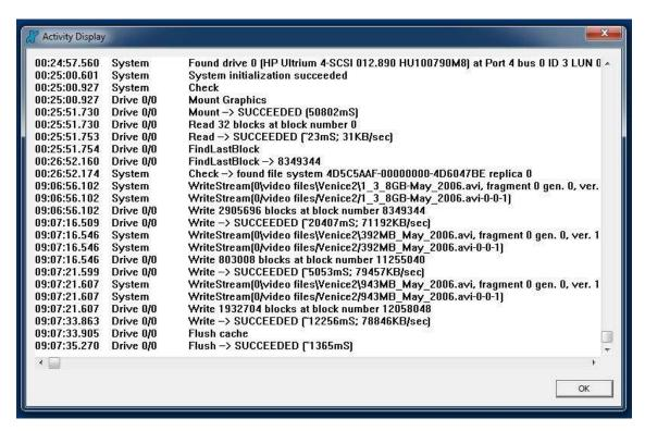
It shows interaction of the archive system with the LTO tape drives and is launched as follows.
